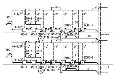
Figure 1: Single-Line Plumbing Riser Diagram
