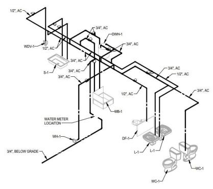
**Figure 2: Axonometric Projection**
