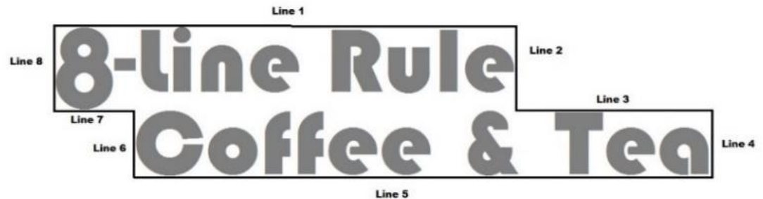
Figure 7100.2: Measuring Building-Mounted Sign Area
