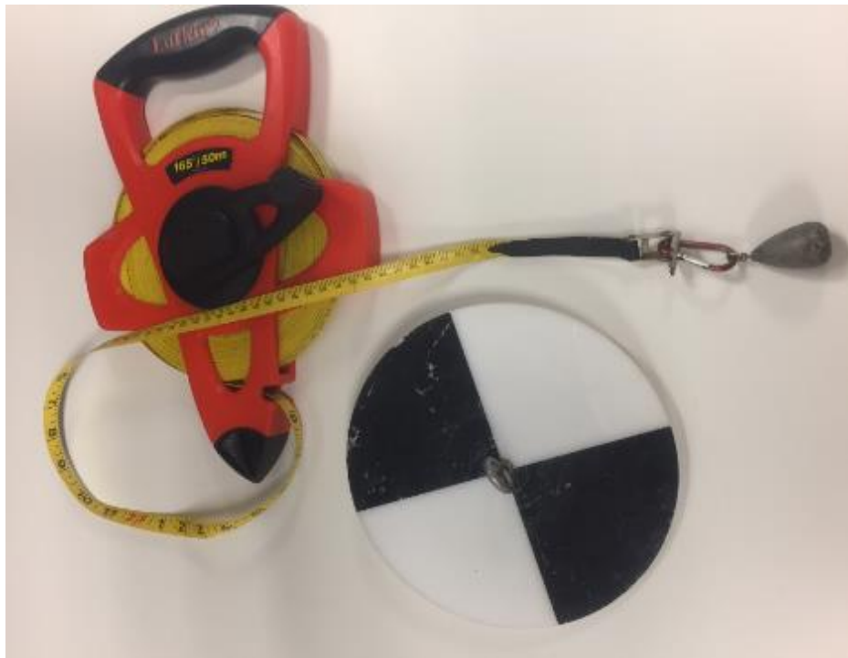
Figure VII.5: 50-Meter Tape measure with cm/mm, Weight and Secchi Disk
