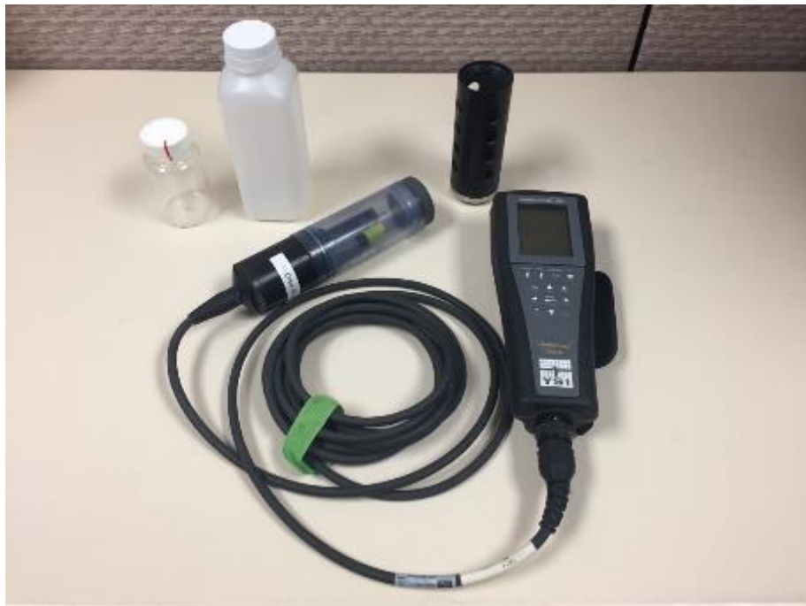
Figure VI.1: Sampling Materials(clockwise from top left: 120ml IDEXX sample bottle, 250ml HDPE sample bottle, YSI multi-parameter water quality sonde)
