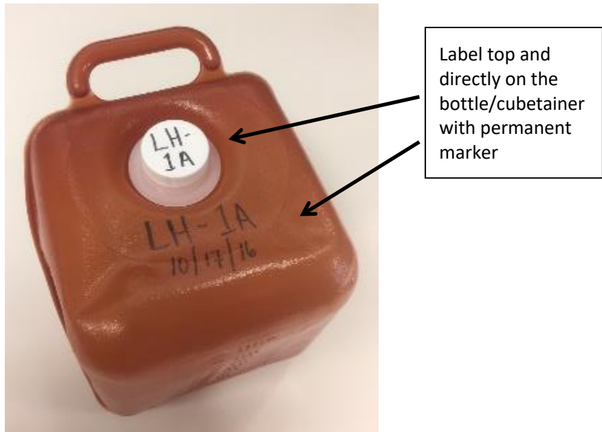
Figure VII.6: One-Gallon/4L Cubetainer Sample Bottle, with Labeling
