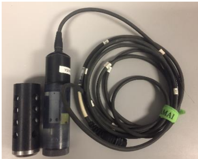
Figure VII.4: YSI Probe, Cable and Guard (with 0.5m Markings)
