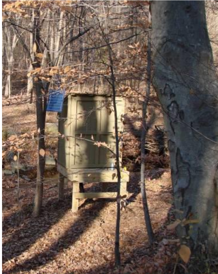
Figure VIII.2: Dead Run Autosampler Shelter
