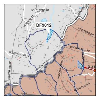
component around 75% of the perimeter of the pond. The proximity of the residence to this pond may become a public safety issue, so careful analysis of water surface elevations of various storm events is required.
