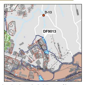
pond to a wetland by removing the existing concrete channels and excavating the bottom area of the pond. Replacing the concrete channels with meandering flow paths through wetland areas will increase detention time, promote uptake of nutrients, removal of pollutants, and settling of sediment.
