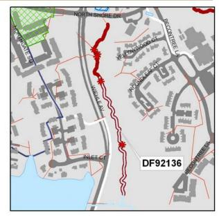
that more closely resembles a natural stream. The outfalls will need to be replaced and the blockage removed. Banks will be stabilized and bed morphology will be improved. Native trees and shrubs will be replaced along the stream banks to provide stability. **Portions of this project may be constructed or superseded by Reston Association work in this stream channel.**
